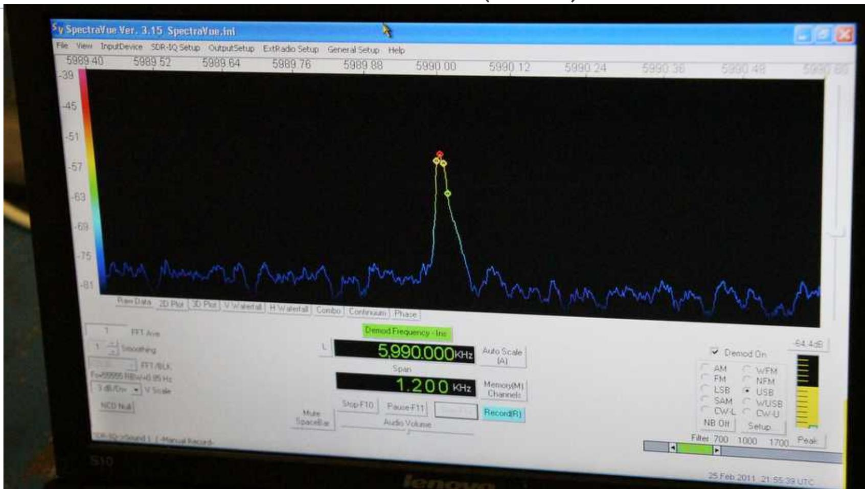
In this case, we see a span of  $\pm 600$  Hz around the Phase Cal “rail”. The Resolution Bandwidth (RBW) is 0.85 Hz and the screen is showing a 40 dB amplitude range.
